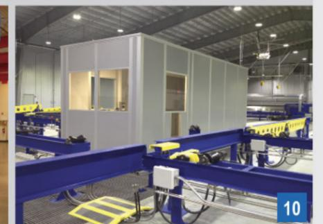
5. Modular buildings can be used to create custom equipment enclosures like this one that houses a laser used to weld small components for the automotive industry. This unit was constructed on top of a steel base frame to enhance portability.
